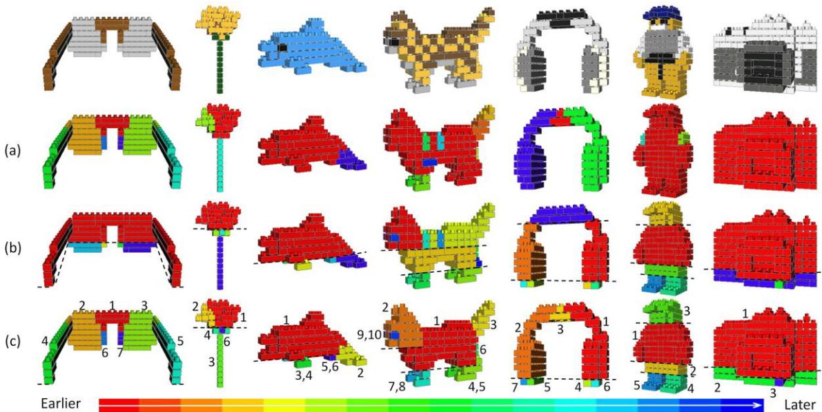
Fig. 5: Generation and ordering of components in different test models (top row). (a) *Block segments* separated at weakly-connected blocks. (b) *Block segments* avoiding *floating blocks*. (c) Final components generated. Assembly order of final components, as marked by numbers, is associated with a specific color in a color map varying from red (built first) to blue (built last).
