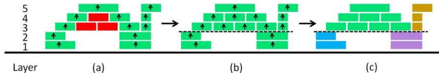
Fig. 2: Segmentation avoiding *floating blocks*. (a) Detecting *floating blocks* (red blocks) along arrows. (b) A *pseudo floor* is inserted between the 2nd and 3rd layers. (c) The model is divided into four *block segments*.
